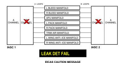
Loss of both B channels effect on BALODS Figure 02–02–20
