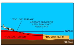
Mode 4B - Unsafe terrain clearance - Approach (gear down) Figure 16-05-13
