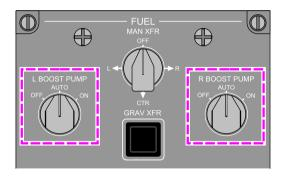
L BOOST PUMP and R BOOST PUMP switches Figure 11–03–2
