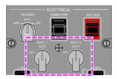
ELEC synoptic page – BATT 1 and BATT 2 switches at AUTO Figure 07–06–13
