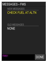
FUEL INSUFFICIENT FOR FINAL AND ALTERNATE
