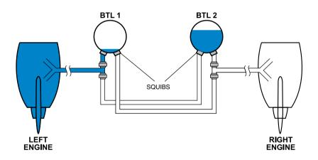
Left engine fire with fire-extinguishing BTL1 discharged Figure 09-02-5
