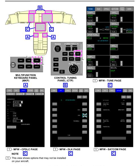
CNS switch with TUNE, DLK, CPDLC, and SATCOM pages Figure 05-09-9
