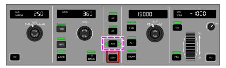
FLIGHT CONTROL PANEL (FCP) - XFR (TRANSFER) SWITCH
