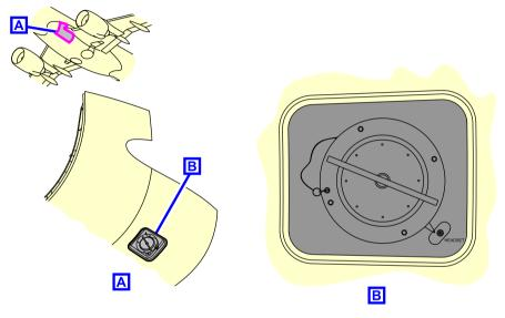
Low Pressure Ground Connection (LPGC) service panel location – Single Jack <23410001D> or <23411001C> Figure 05–04–18
