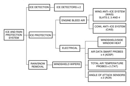
Ice and rain protection system (schematic)
