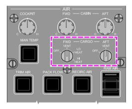
AIR panel – FWD CARGO switch and AFT CARGO switch Figure 02–03–31
