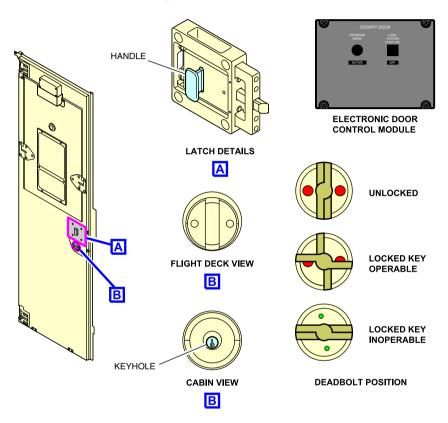
Electronic door control module – latch and deadbolt Figure 06–06–8
