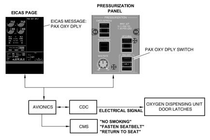
Manual deployment schematic <33200010C> Figure 17–02–13
