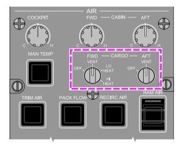
AIR panel – FWD CARGO switch and AFT CARGO switch Figure 02–03–16
