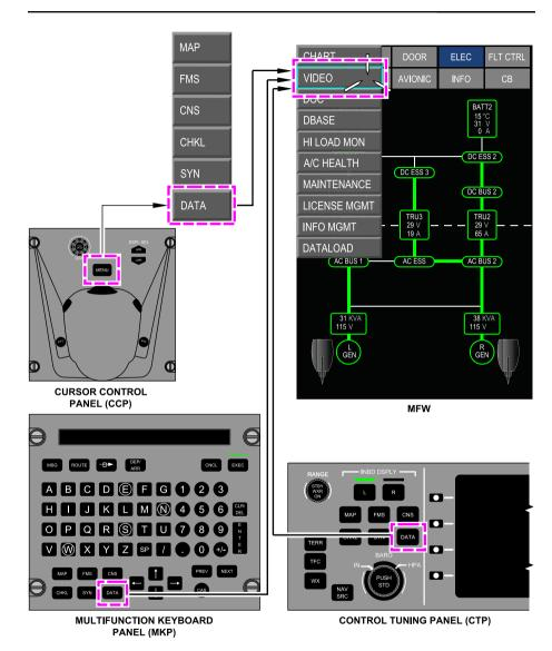
Flight deck door surveillance system – Video access Figure 06–06–5
