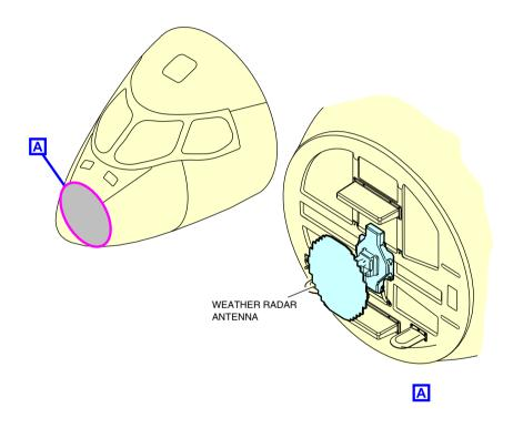
MultiScan weather radar antenna Figure 16–06–1
