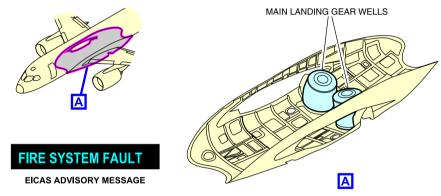
Main landing gear overheat detection loops Figure 09–06–1
