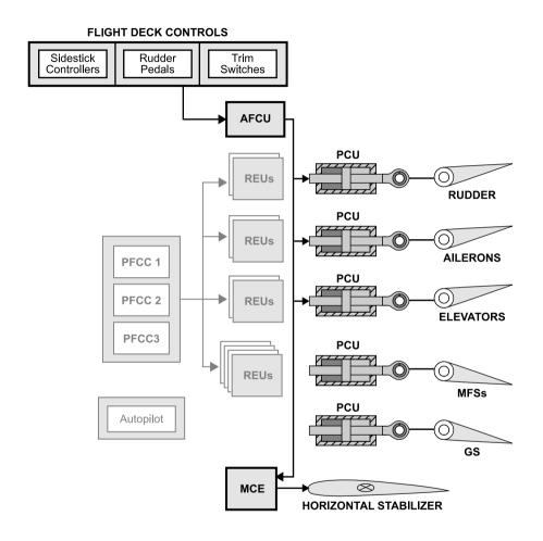
Alternate Flight Control Unit (AFCU) logic Figure 10–02–5
