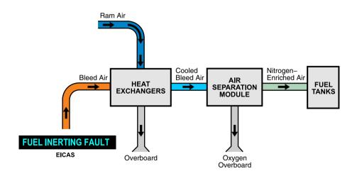
Fuel inerting system schematic Figure 11–07–1
