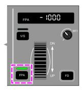
Flight Control Panel (FCP) – FPA (Flight Path Angle) switch Figure 03–06–16
