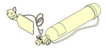
Portable oxygen cylinders and masks Figure 17–03–2
