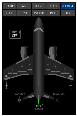
Primary Flight Control Computer (PFCC) switches Figure 10–02–3
