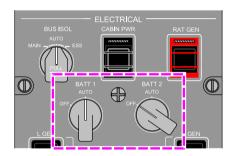
ELEC synoptic page – BATT 1 switch at AUTO and BATT 2 switch at OFF Figure 07–06–12
