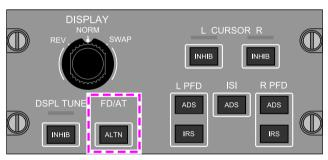
REVERSION SWITCH PANEL (RSP)-FD/AT ALTN (ALTERNATE) SWITCH
