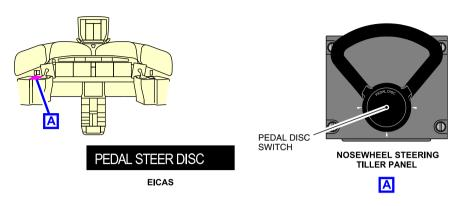
Rudder pedal disconnect Figure 14–03–4
