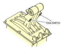
THROTTLE QUADRANT ASSEMBLY (TQA) - TOGA SWITCHES
