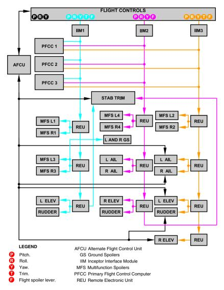
Fly-By-Wire (FBW) system schematic Figure 10-02-2
