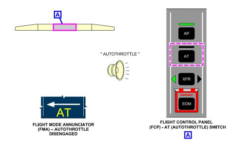
Autothrottle (AT) system disengagement – AT switch Figure 03–06–11
