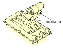
THROTTLE QUADRANT ASSEMBLY (TQA) - TOGA SWITCHES
