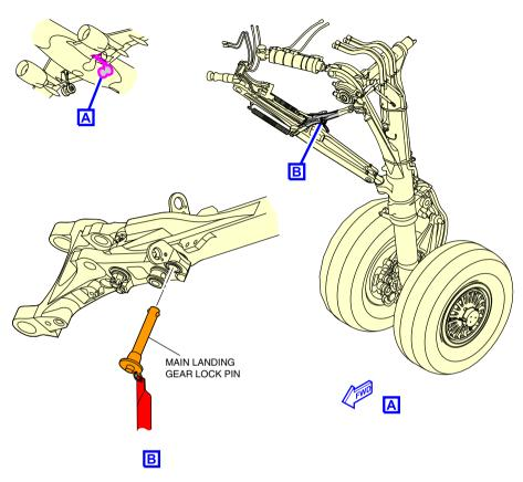
Main landing gear lock pin Figure 01–02–4
