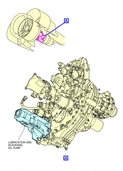
Main gearbox – Lubrication and scavenge oil pump Figure 18–07–5
