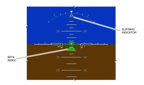
ADI – Slip/skid indicator and beta index (OEI with slats/flaps retracted) Figure 08–03–9
