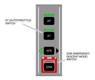
FCP – AT (Autothrottle) and EDM (Emergency Descent Mode) switch Figure 03–05–5
