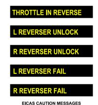
Thrust reversers deployment malfunctions Figure 18–02–6
