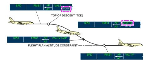
VNAV Path (VPATH) – Altitude Constraint Figure 03–02–37
