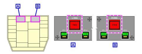
Left and right engine fire switch/light Figure 12–02–12
