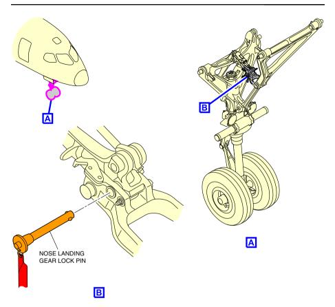
Nose landing gear lock pin Figure 01–02–5
