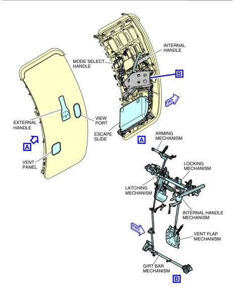
Passenger and service door mechanisms Figure 06–02–7
