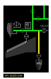
AIR synoptic page – Engine and APU bleed leak indications Figure 02–02–15
