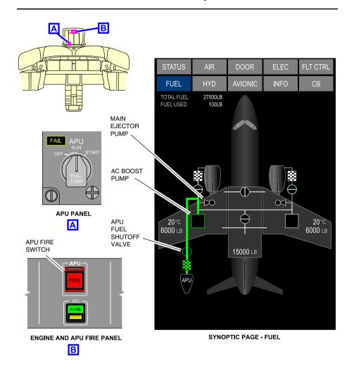
APU fuel feed shutoff valve controls Figure 11–03–7
