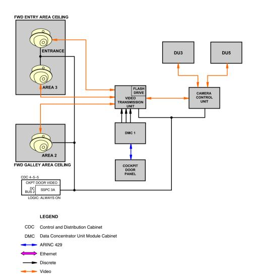
Flight deck door surveillance system diagram <23730002C> Figure 06–06–4
