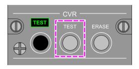
CVR panel – TEST switch Figure 19–05–2
