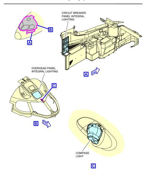
Overhead panel, circuit breaker panels, and compass lights Figure 15–02–3
