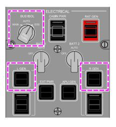
ELEC synoptic page – BUS ISOL switch at ESS, L GEN ON and R GEN ON Figure 07–06–28
