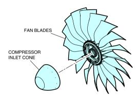
Compressor inlet cone and fan blades Figure 18–03–2
