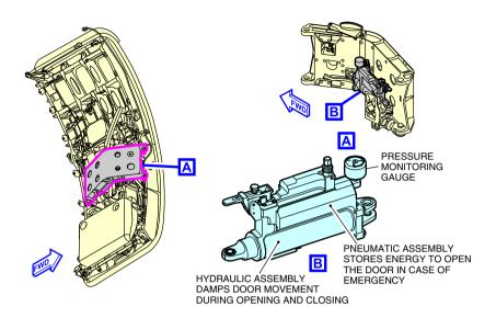
Main door opening assist mechanism location Figure 06–02–5
