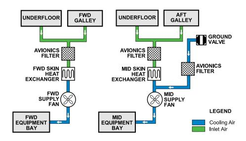
Avionics cooling system Figure 02–03–18
