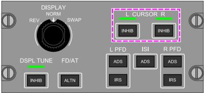
REVERSION SWITCH PANEL (RSP) - L AND R CURSOR INHIBIT SWITCHES
