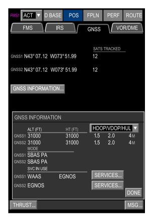
POS soft switch - GNSS Tab - GNSS INFORMATION window Figure 16-03-5
