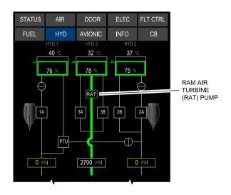
Hydraulic system No. 3 – Ram Air Turbine (RAT) pump Figure 12–03–9
