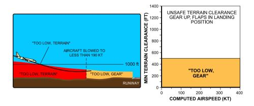
Mode 4A – Unsafe terrain clearance – Approach (gear not down) Figure 16-05-12
