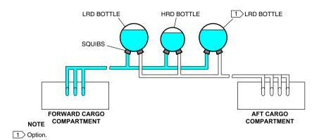
Cargo compartment fire–extinguishing bottles Figure 09–04–6
