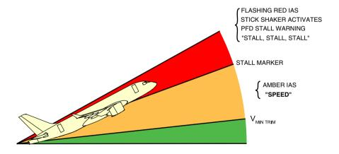
High Angle-of-Attack protection direct mode Figure 10-02-25
