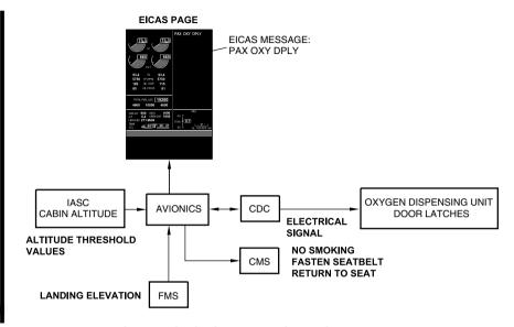
Automatic deployment schematic <33200010C> Figure 17–02–12
