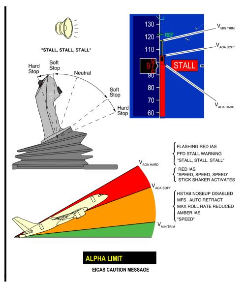
High Angle-of-Attack protection normal mode Figure 10-02-11
