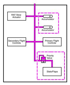
Hydraulic System no. 3 – Accumulators and Priority Valve Figure 12–03–8
