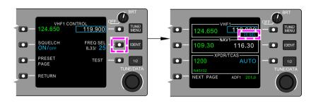
CTP – Spacing selection on the VHF1 CONTROL or VHF2 CONTROL pages Figure 05–03–18
