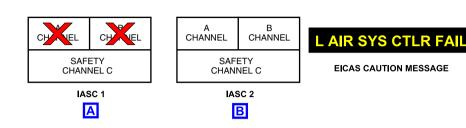
IASC complete failure effect on the bleed air valves Figure 02–02–11
