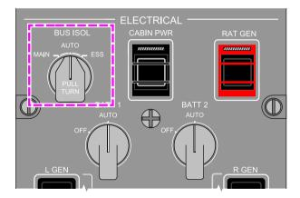
ELEC BUS ISOL MAIN ELEC BUS ISOL ESS
