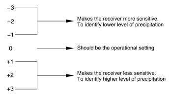
Radar gain control setting Figure 16–06–14
