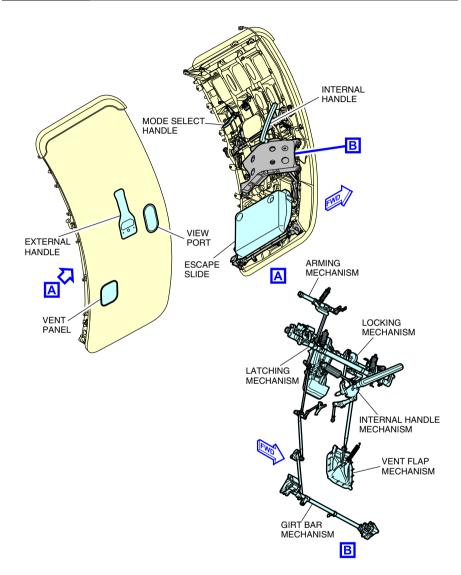
Passenger and service door mechanisms Figure 06–02–2
