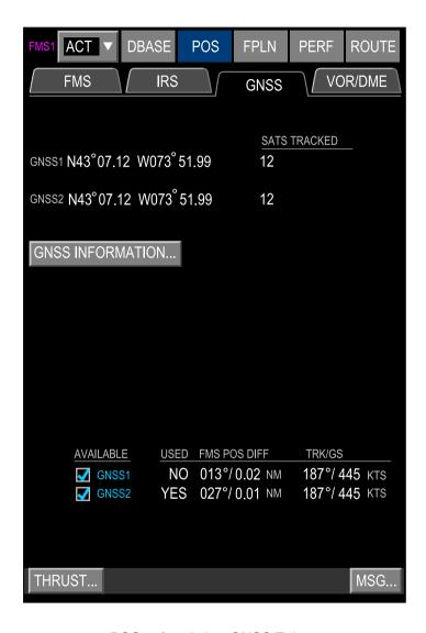
POS soft switch - GNSS Tab Figure 16-03-4
