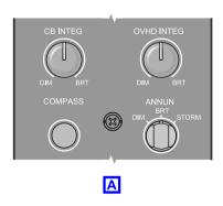
Overhead panel, circuit breaker panels, and compass lights controls Figure 15–02–4
