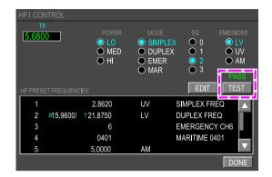
TUNE page – HF1 CONTROL window – TEST soft switch <23129001C> Figure 05–03–76
