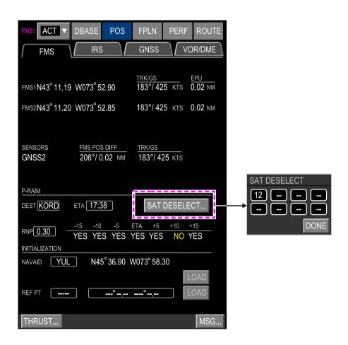
POS soft switch - FMS tab - SAT DESELECT window Figure 16-03-9
