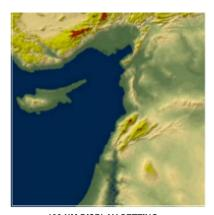
100 NM DISPLAY SETTING MEDIUM INTENSITY YELLOW FOR TERRAIN ≤ 500 FEET BELOW TO < 2000 FEET ABOVE AIRCRAFT ALTITUDE.
