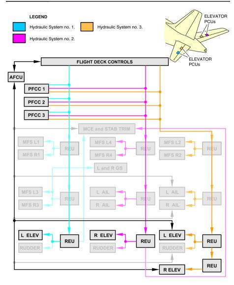
Elevator system schematic Figure 10–03–5
