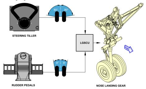
Nosewheel steering system Figure 14–03–1
