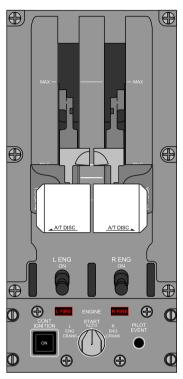
THROTTLE QUADRANT ASSEMBLY (TQA) AND ENGINE PANEL
