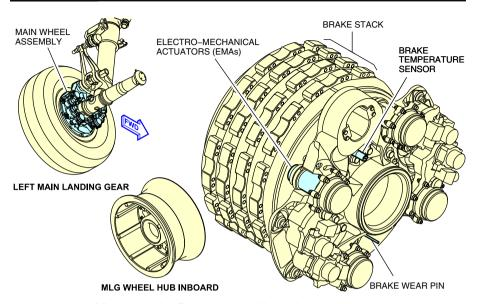
Main wheel – Brake assembly and tire assembly Figure 14–04–6
