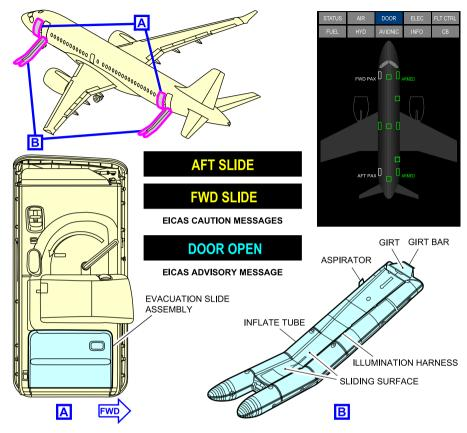
Main door slide deployment mechanism <52201001D> Figure 06–03–2
