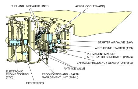
Engine accessible components (left side) Figure 18–02–2
