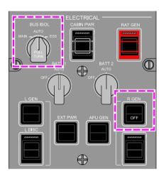
ELEC synoptic page – BUS ISOL switch at AUTO and R GEN OFF Figure 07–06–26
