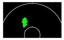
RADAR RETURN OF OCEANIC THUNDERSTORM IF SAME TILT, GAIN AND PULSE WIDTH ARE UTILIZED.
