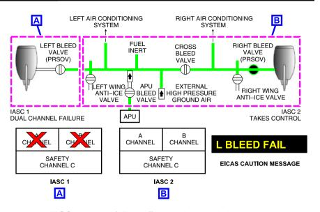
IASC complete failure effect on the bleed air valves
