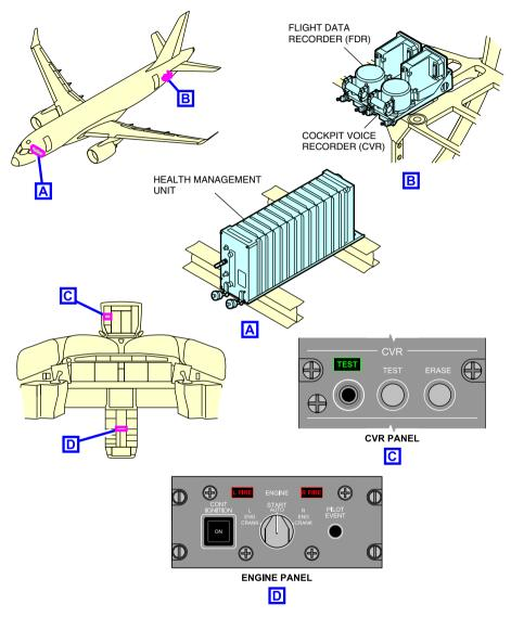
Recording system location and controls Figure 19–01–1
