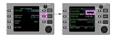
CTP – Channel spacing selection on the VHF1 or VHF2 CONTROL pages <31000008C>
