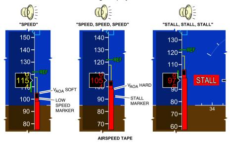
ADI – Airspeed tape – Low speed indications – Normal mode Figure 08–03–32
