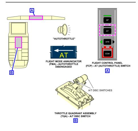
Autothrottle (AT) system disengagement Figure 03–05–6
