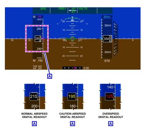
ADI – Airspeed tape – Airspeed digital readout Figure 08–03–22
