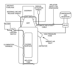
Main door slide deployment mechanism schematic Figure 06–03–1
