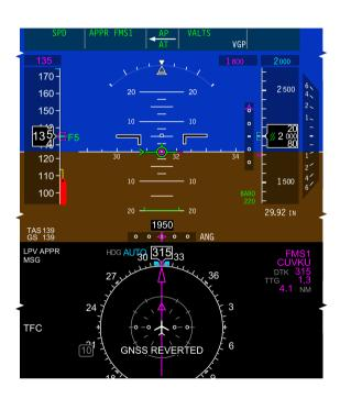
Failure indications after LPV APPR active Figure 22–03–37
