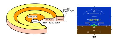
Terrain Floor Clearance (TFC) – Alert envelope Figure 16-05-25
