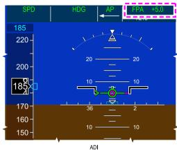
Flight Path Angle (FPA) – Positive angle Figure 03–02–22
