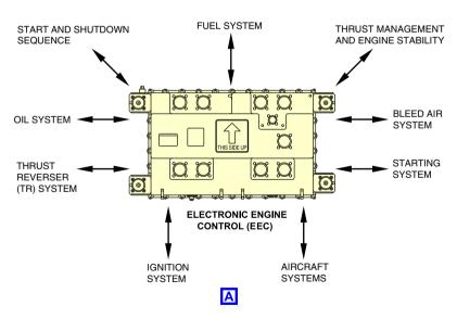
Electronic engine control (EEC) interaction Figure 18–03–11
