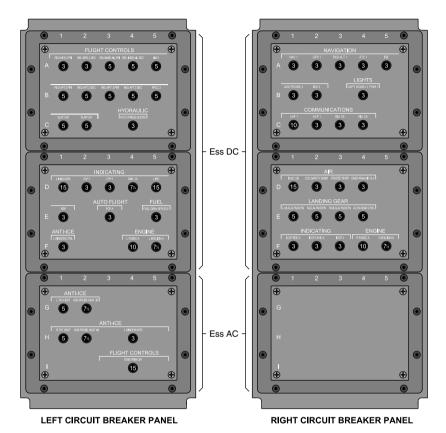
Flight deck circuit breaker panels Figure 07–05–4
