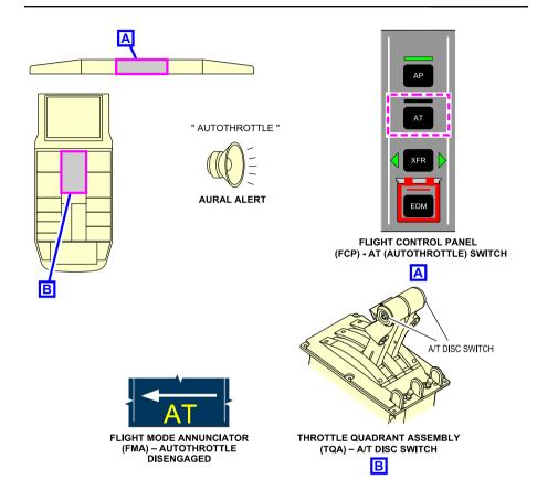
Autothrottle (AT) system disengagement – A/T DISC switch Figure 03–06–19
