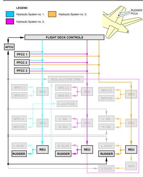
Rudder system schematic Figure 10–03–7
