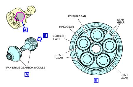
Fan Drive Gear System (FDGS) module Figure 18–03–3
