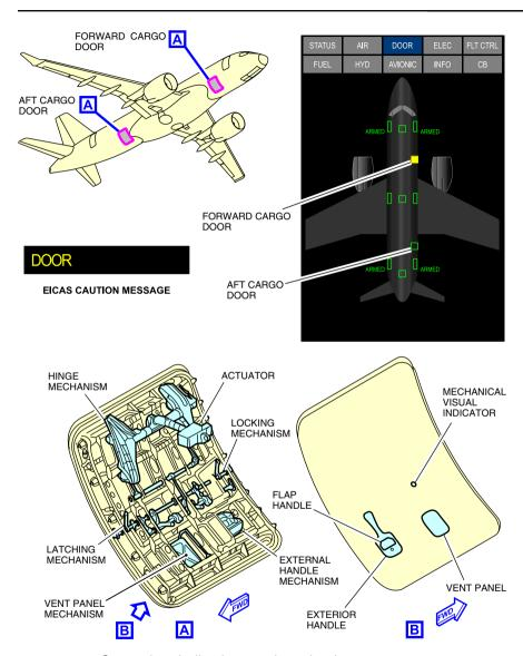
Cargo door indications and mechanisms <52201001D> Figure 06–04–2
