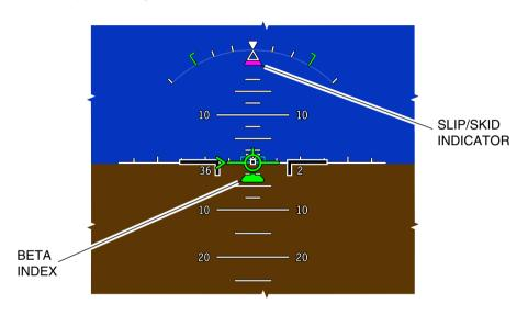
ADI – Slip/skid indicator and beta index (OEI at takeoff and weight–off–wheels)
