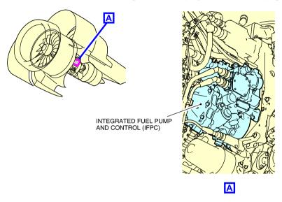
Integrated Fuel Pump and Control (IFPC) Figure 18–05–3
