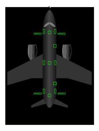
DOOR synoptic page – On ground or in flight – All doors are latched and locked <52201001D>
