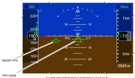
GHOST FPV INDICATES AIRCRAFT FLIGHT PATH OUTSIDE THE CAGE FPV AREA
