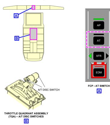
Autothrottle (AT) system controls Figure 03–05–1
