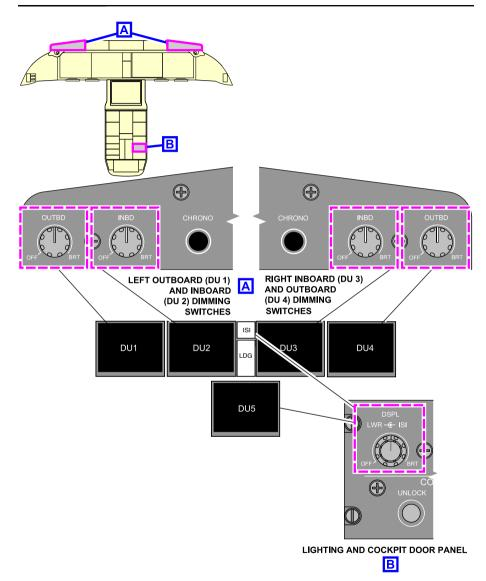
Display dimming switches Figure 08–02–16
