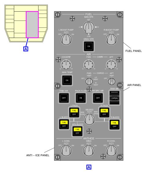
Right inboard overhead module Figure 01–02–25
