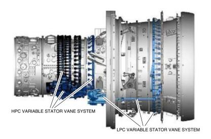
Compressor variable stator vane system Figure 18–05–7
