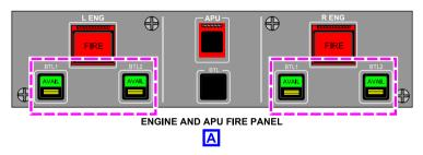
Engine and APU fire panel – ENG FIRE BTL switches Figure 09–08–5
