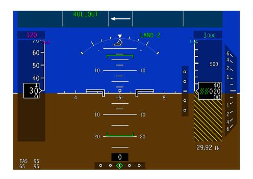
ROLLOUT mode less than 30 kt ground speed Figure 03–04–9
