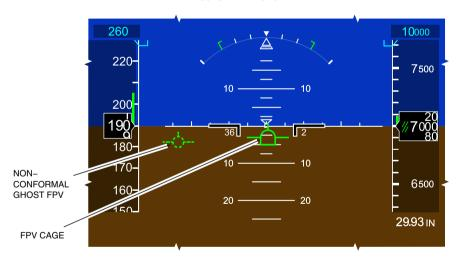
NON-CONFORMAL GHOST FPV INDICATES AIRCRAFT FLIGHT PATH OUTSIDE OF THE CAGE FPV AREA LIMITS
