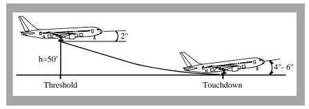
Typically, the pitch attitude increases slightly during the actual landing, but avoid over-rotating. Do not increase the pitch attitude after touchdown; this could lead to a tail strike.
