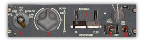
The Autopilot control unit is located in the radio stack, lower right side of the captain. There are 2 knobs, 2 levers and 2 switches that operate the SP-50.
