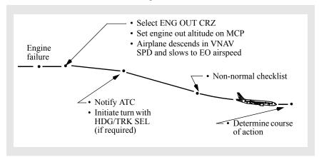
**Note:** If the airplane is at or below maximum engine out altitude when an engine becomes inoperative, select and execute the EO CRZ page and maintain engine out cruise speed.
