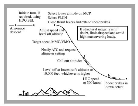
If the descent is performed because of a rapid loss of cabin pressure, crewmembers should place oxygen masks on and establish communication at the first indication of a loss of cabin pressurization. Verify cabin pressure is uncontrollable, and if so begin descent. If structural damage exists or is suspected, limit airspeed to current speed or less. Avoid high maneuvering loads.
