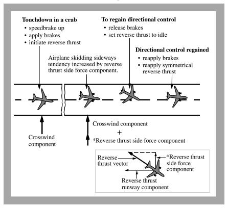
This figure shows a directional control problem during a landing rollout on a slippery runway with a crosswind. As the airplane starts to weathervane into the wind, the reverse thrust side force component adds to the crosswind component and drifts the airplane to the downwind side of the runway. Also, high braking forces reduce the capability of the tires to corner.
