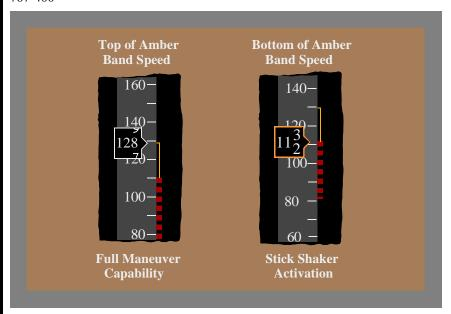
Minimum maneuver speeds (displayed as the top of the lower amber band) should not be confused with flap maneuver speeds. Flap maneuver speeds are based on airplane weight, while the minimum maneuver speed is based on airplane angle of attack and current airspeed. These speeds provide independent means to ensure that the current airspeed provides at least full maneuver capability for terminal-area maneuvering.
