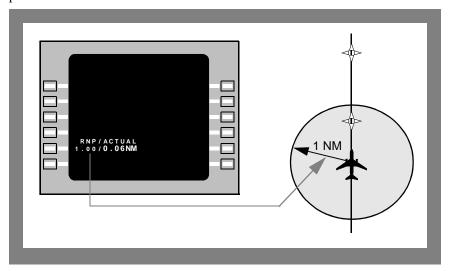
Oceanic RNPs are generally 4.0 or higher. Domestic en-route RNAV operations depend on the availability of radio updating (DME-DME) sources to support domestic RNPs. The following domestic RNP operations are fully supported by any Boeing FMC with DME-DME or GPS updating active:
