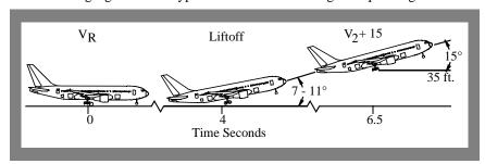
Retract the landing gear after a positive rate of climb is indicated on the altimeter. Retract flaps in accordance with the technique described in this chapter.
