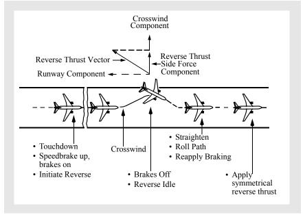
This figure shows a directional control problem during a landing rollout on a slippery runway with a crosswind. As the airplane starts to weathervane into the wind, the reverse thrust side force component adds to the crosswind component and drifts the airplane to the downwind side of the runway. Main gear tire cornering forces available to counteract this drift are at a minimum when the antiskid system is operating at maximum braking effectiveness for the existing conditions.
