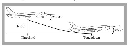
Typically, the pitch attitude increases slightly during the actual landing, but avoid over-rotating. Do not increase the pitch attitude after touchdown; this could lead to a tail strike.
