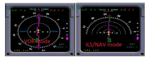
The navigation display is situated directly to the right of the PFD. The Airbus ND can display a myriad of information. The ND can display: TCAS information, ILS deviation, as well as graphical and textural information related to flight management. The different modes of the ND can be displayed using the EFIS control panel which is pictured below.
