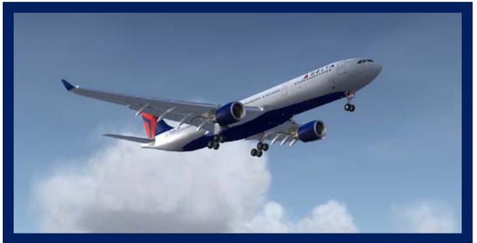
Maintain 180 KIAS until glide slope intercept occurs or you reach a point 10 NM from the runway. At this point, reduce your target speed to 160 KIAS deploying flaps to FULL. Lower the landing gear and turn on the taxi light.
