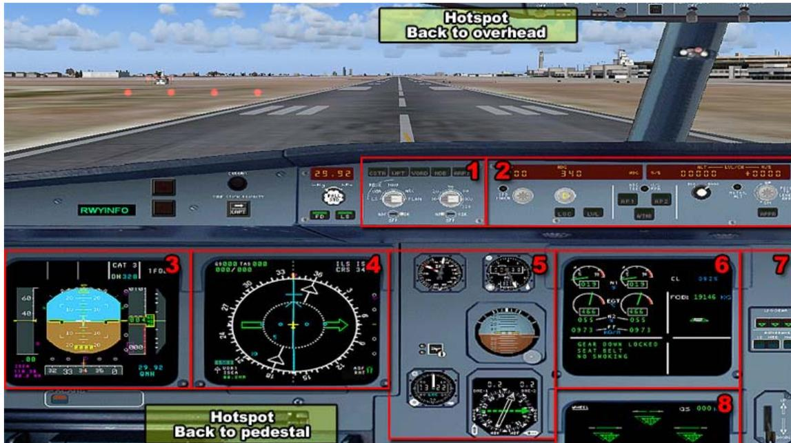
1. **Electronic Flight Instrument Systems (EFIS) control panel.** This panel is used to control the data displayed on the Navigation Display (ND).
