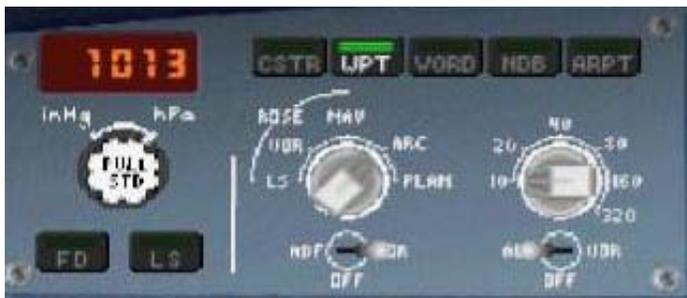
**EFIS Control Panel:** This is where you will make selections for the various ND display views using the selector knobs for system
