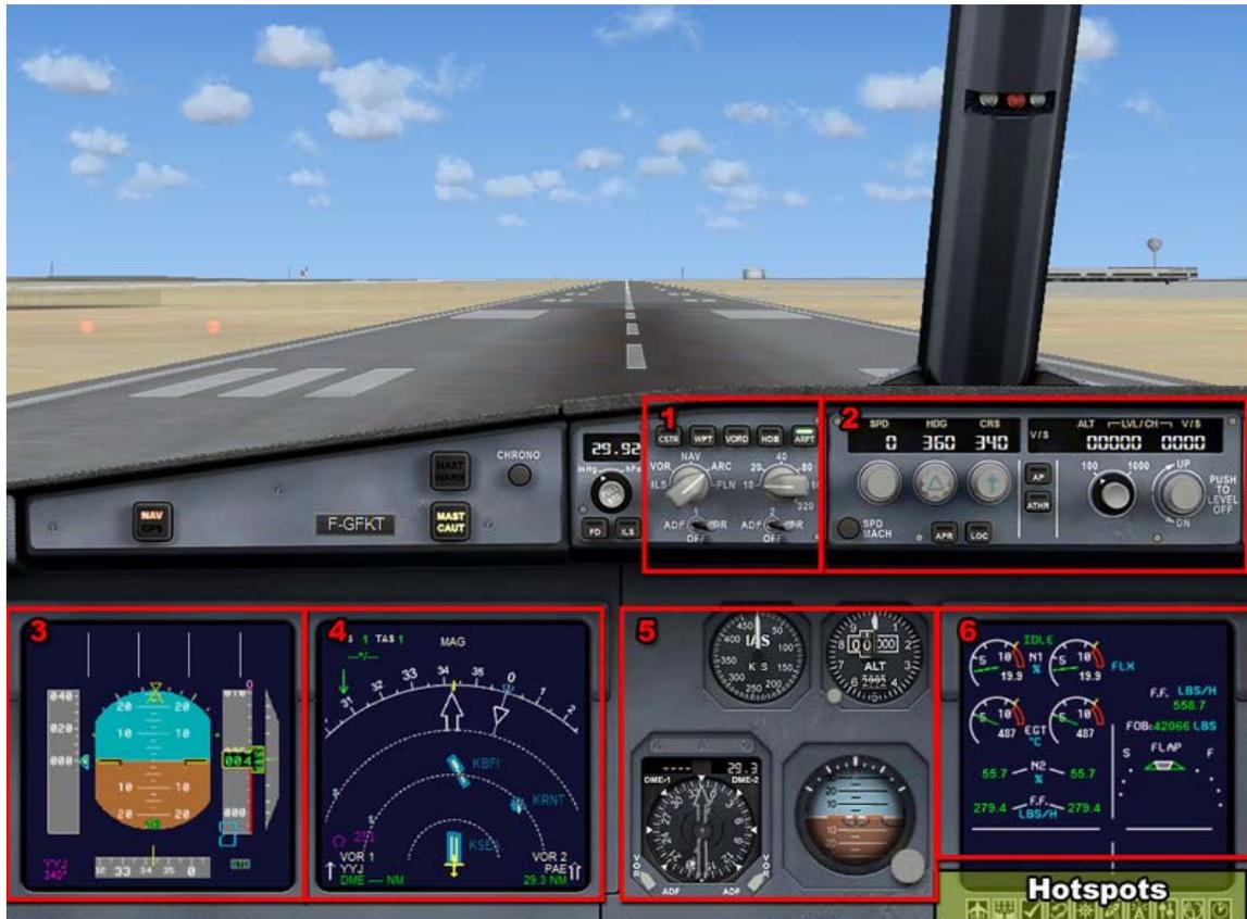
1. **Electronic Flight Instrument System (EFIS) control panel.** This panel is used to control the data displayed on the Navigation Display (ND).
