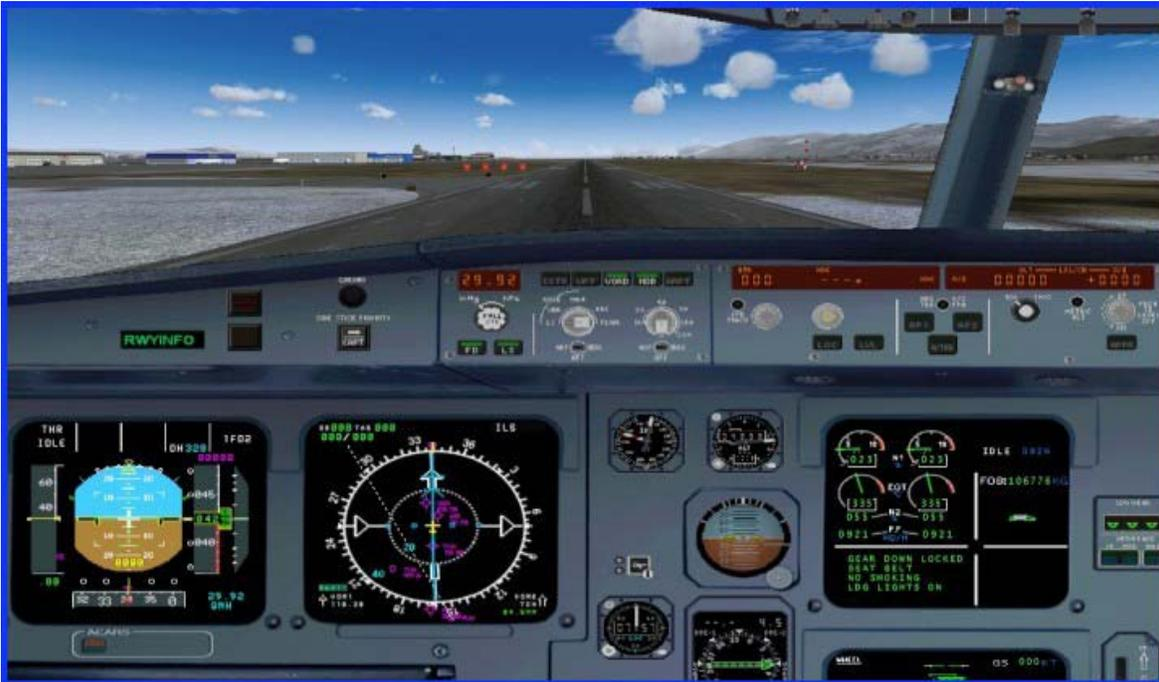
Using the DVA A330 fleet installer aircraft, you will be working in a two dimensional environment. Above is the instrument panel of the DVA Airbus A330-200. Immediately you will notice that most of your gauges are found on the electronic displays, with only a few standby gauges in case of system failure. Let's work from left to right as we review what we are looking at:
