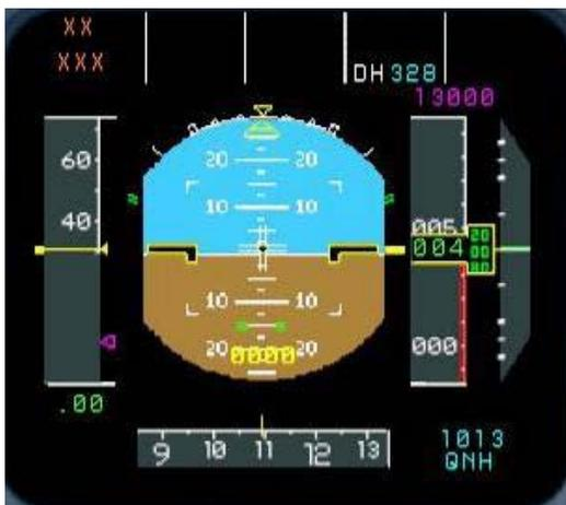
Primary Flight Display (PFD)-This is the outboard display unit (DU). Within the PFD display unit we have the electronic speed tape on the left and altitude ribbon on the right. Sandwiched between the two is the Electronic Attitude Direction Indicator (EADI). On the bottom is an electronic compass
