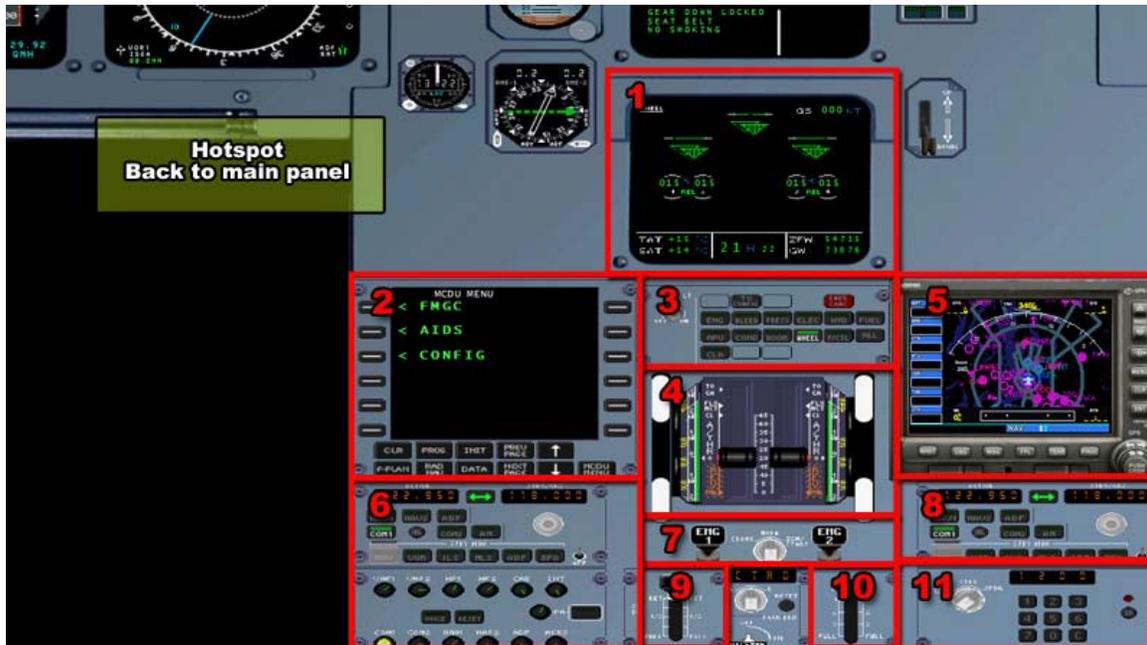
**System Display (SD).** The lower screen of the Electronic Centralized Aircraft Monitor (ECAM) featuring information related to the various aircraft systems.
