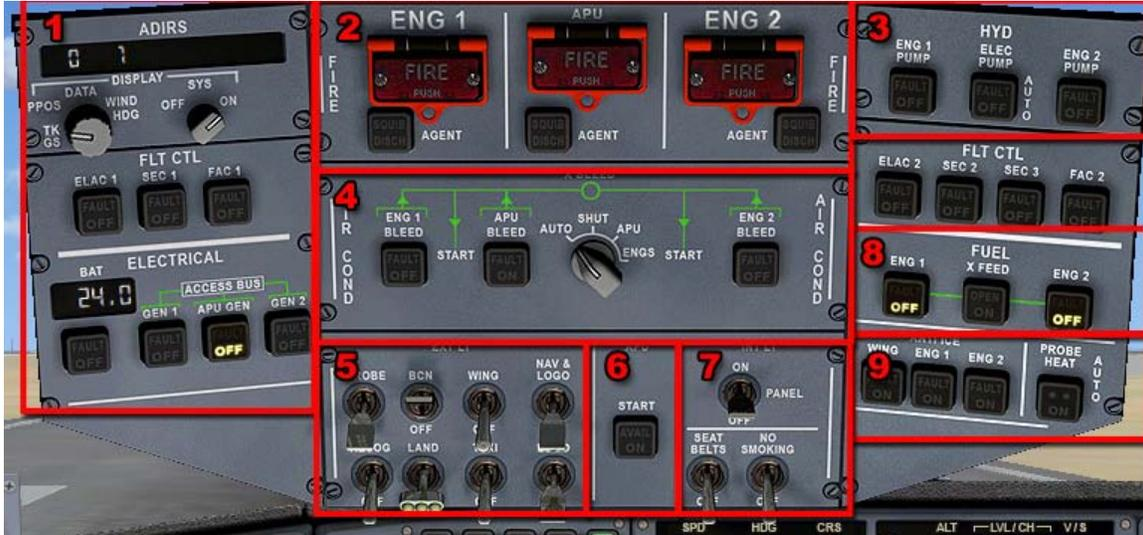
**Air Data and Inertial Reference System Control Display Unit (ADIRS CDU).** These switches and displays are used to manage the aircraft's primary navigation system.
