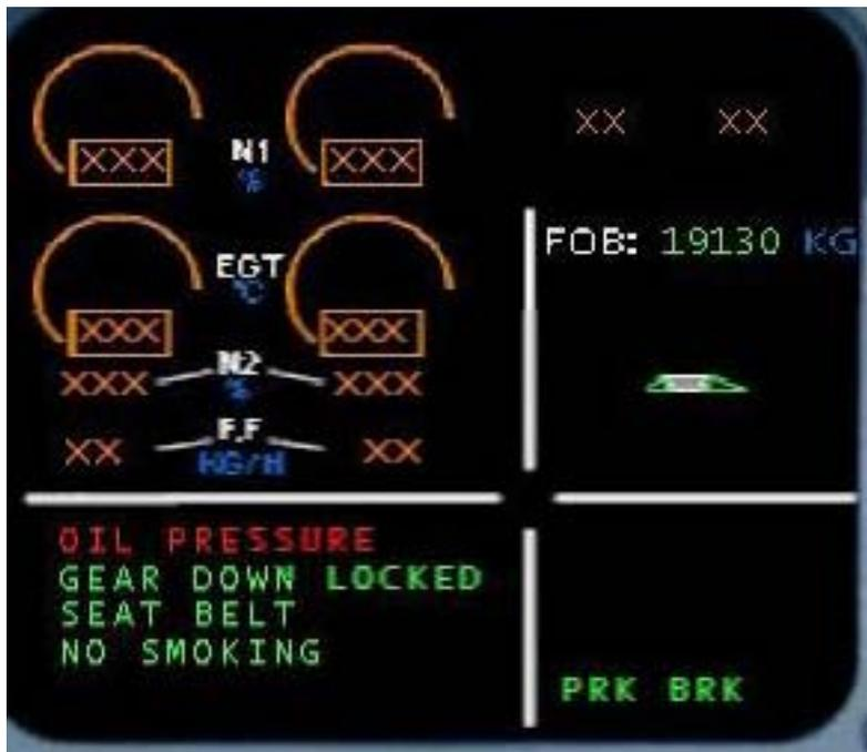
The lower left quarter shows takeoff and landing checklists and presents you with other information during flight, such as reminders for landing lights and No Smoking and Seatbelt signs. The lower right quarter shows auto brake settings.
