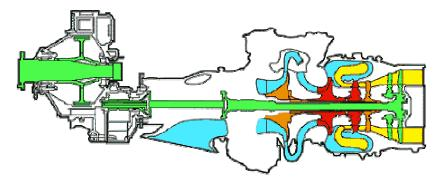
A turboprop engine, on the other hand, is essentially a jet turbine. Instead of driving a fan like a turbofan engine, the turbine spins the propeller shaft, propelling large amounts of air outside the engine altogether. In many ways, a turboprop is just a turbofan engine where the fan has fewer blades and is not contained within the engine nacelle.
