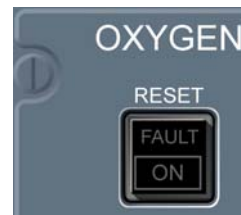
OXYGEN MAINTENANCE Panel
